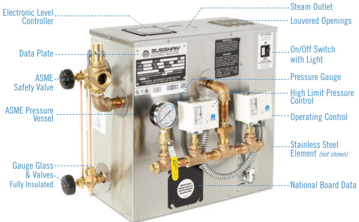
TYPICAL BOILER ARRANGEMENT
